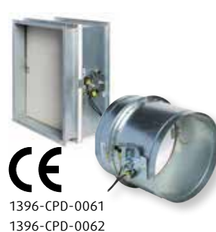
Fire dampers to ATEX Enviroment EI60/90/120S tested according to EN 1366- 2 conform with directive 94/9/EC for classification Ex II 2/- G c IIB
