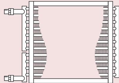
**PBT** Horizontal Airflow - Opposite End Connectors
