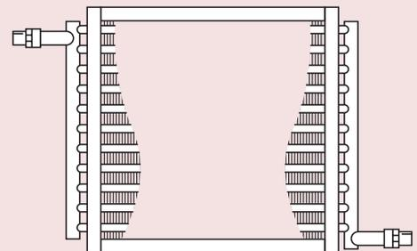
**PBT** Horizontal Airflow - Vertical Tubes
